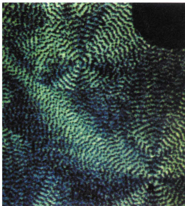
Fig. 4 Texture of ( S )-Pc(8,2) observed between crossed polarizers at room temperature
